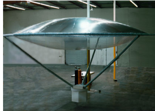
Figure 4: Inflatable Reflector Development at L'Garde
