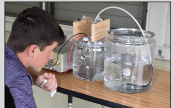
Designed by Nolan and Ryan Pries, the electrolysis device captures hydrogen in a submerged flask.
